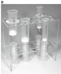
Figure 3 Setup of NucleoBond® Xtra Columns with the NucleoBond® Xtra Combi Rack A: Setup for clarification, loading, and first washing step; B: Setup for elution.
